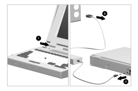
Figure 5-4. Disconnecting the Computer
